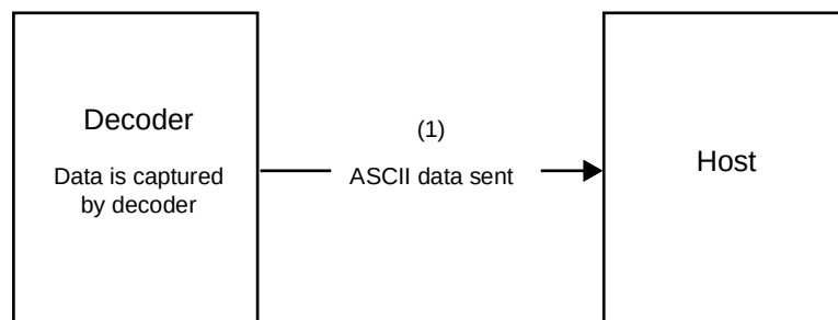
Figure 9-4 ACK/NAK Disabled and Unpacketed ASCII Data
